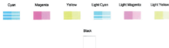
Figure 9-2 Example of color blocks with defects
